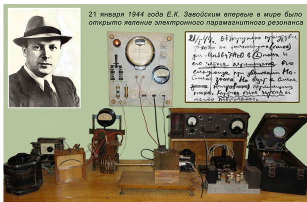
Fig. 3 The device made by E.K. Zavoisky, which made it possible, for the first time, to detect EPR signals. Reconstructed by I.I. Silkin in the Memorial Laboratory of Zavoisky at Kazan Federal University. Photo by I.I. Silkin, the curator of the Memorial Laboratory
